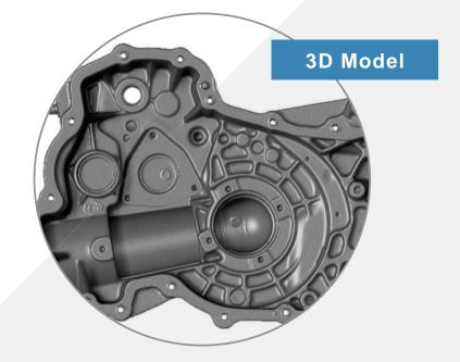
3D scanners can be used to get complete or partial 3D measurements of any physical object. The majority of these devices generate points or measures of extremely high density when compared to traditional "point-by-point" measurement devices. OBJECTS ARE USUALLY SCANNED IN 3D FOR
